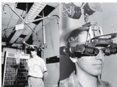
图2 “The Sword of Damocles”原型头显设备
