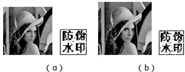
(a)添加高斯噪声后提取水印( NC = 0.9732 ) (b)添加椒盐噪声后提取水印( NC = 0.9463 )
